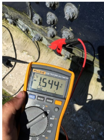
(Left) Greatario installed its first permanent glass coated tank in Midhurst in 1986. (Top right) Anodes installed on the glass fused to steel floor can be tested from the outside of the tank using a multi-meter +CSE per NACE requirements, while the tank is in service (bottom right).
